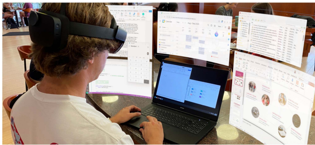
Fig. 2. User working at a cafe in study 1: hybrid canvas display expands a laptop monitor with virtual space around it.
