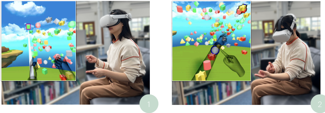
Figure 4: An example of a user using the mid-air surface for object selection (1) and the on-body surface for object selection (2).
