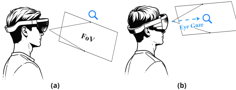
Figure 1: (a) The neutral head position while wearing the HoloLens2. The search icon is placed at the body-fixed top position. (b) The user moves their head and eye gaze to align with the search icon for activation of the virtual keyboard in both UPDWELL and UPDWELLFREE.
