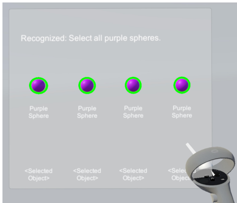
Figure 3: Draggable panel of AssistVR which displays the recognized speech and a list of names and 3D previews of all selected objects. Here, the user states ‘Select all purple spheres’, and all four purple spheres in the scene are selected.
