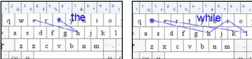
Figure 3.2. The words the and while mapped onto a QWERTY software keyboard layout.
