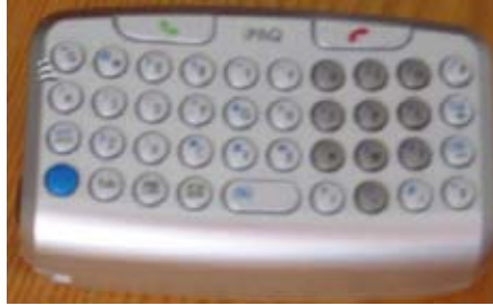
Figure 6.1. A thumb keyboard. The keys have a diameter of 8 mm.
