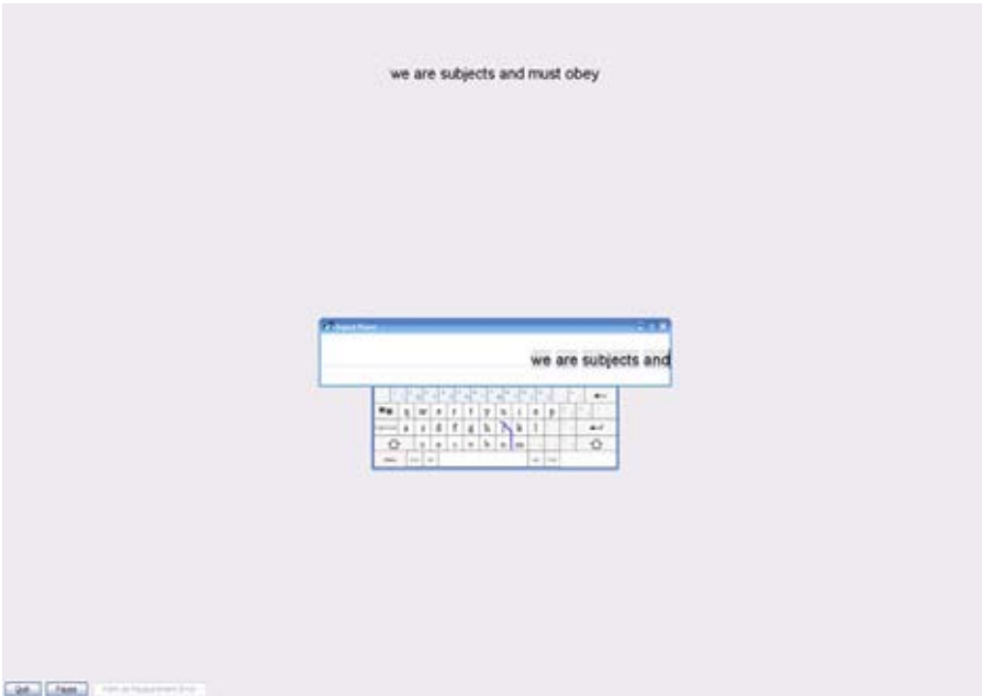
Figure 3.34. The experiment software interface in the shape writing (QWERTY) condition (running on a computer tablet). Participants were encouraged to move the software keyboard to a comfortable position.
