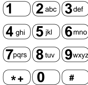
Figure 6.2. The ISO/IEC 9995-8:1994 standard telephone keypad layout.
