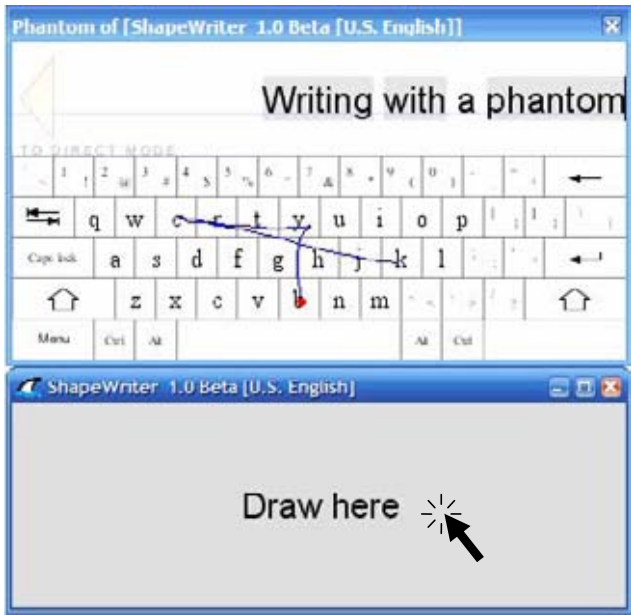
Figure 3.17. Example of writing with a phantom keyboard. The user is in the process of writing the word keyboard .
