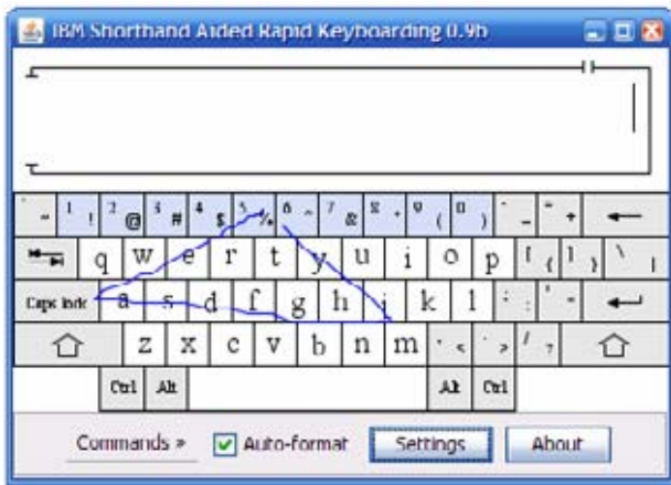
Figure 3.6. Shape writing using the QWERTY keyboard layout. The user’s input in the figure will be recognized as the word that .
