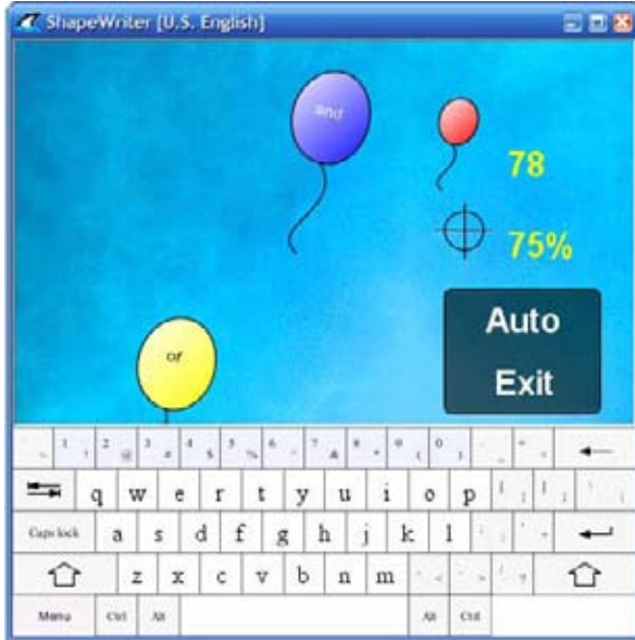
Figure 3.22. The shape writing practice game. The score next to the balloon icon indicates how many words that were successfully inputted (in the figure 78). The percentage next to the crosshair icon shows the accuracy (in the figure 75%). By selecting the AUTO option the system automatically pen-gestures the currently shown words.
