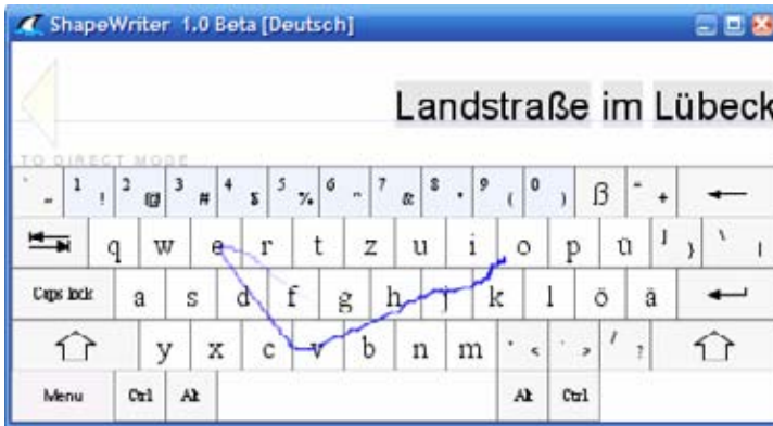
Figure 3.23. Writing German words with continuous shape writing on the QWERTZ software keyboard layout.
