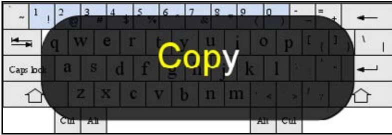
Figure 5.4. The system has recognized the command Copy and overlays it on the keyboard. The shortest acronym the user has to articulate is drawn in a distinct yellow color.
